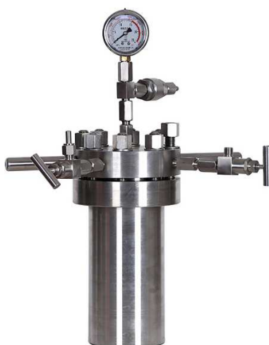
Figure 4. Type of autoclave used to perform the experiments.
