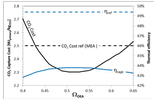
Figure 2: Evolution of the  $\text{CO}_2$  capture cost (left-hand side scale, in black) and the thermal efficiency (right-hand side scale, in blue) of the OEASTIG cycle as a function of the OEA quality ( $\Omega_{\text{OEA}}$ ). Comparison with reference cost of  $\text{CO}_2$  capture (reference value of the post-combustion capture process by MEA (monoethanolamine)-absorption).
