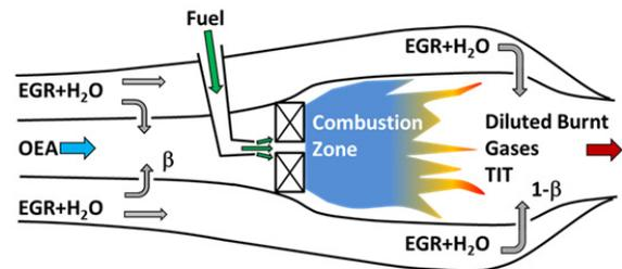
Figure 4: Scheme of the distribution of Fuel, OEA and diluting gases (EGR and H<sub>2</sub>O) in the OEASTIG combustion chamber.
