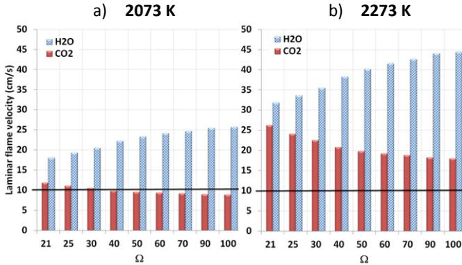
Figure 9: Calculated flame velocities, as a function of  $\Omega$ , i.e. for the conditions listed in table 4 : a) for  $T=2073\text{K}$ ; b) for  $T=2273\text{K}$ . The case with  $\text{H}_2\text{O}$  as diluent is shown in blue and that with  $\text{CO}_2$  as diluent in red.
