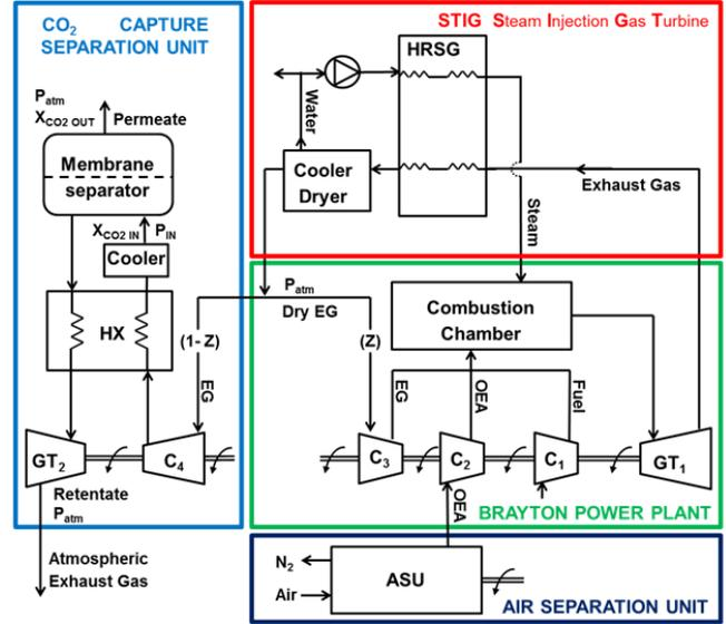
Figure 1: Scheme of the  $\text{CO}_2$  capture hybrid process.
